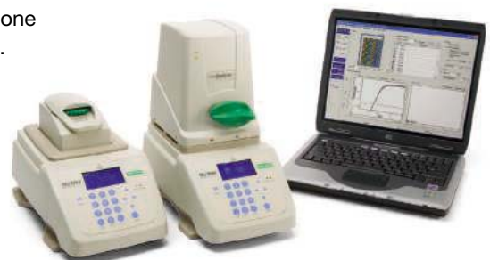
MJ Mini cycler — 18 x 32 x 20 cm; 4 kg MiniOpticon system — 18 x 32 x 33 cm; 8 kg
